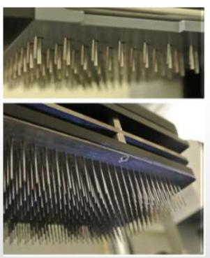
Large scale cleaning - high pressure water jets for devices with lumens
